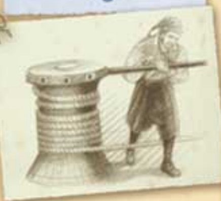
The capstan is a type of winch or windlass that is used to raise the anchor.
