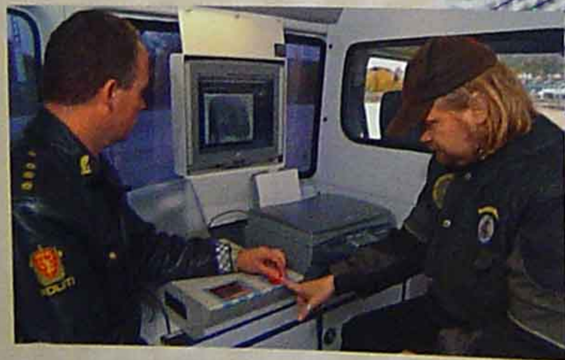
▲ When a suspect (right) is arrested, their prints are taken. In the past fingers were inked and prints placed on cards. Today, many law enforcement forces scan the suspect's fingerprints electronically so that they can be processed immediately.
