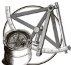
Compass and sextant These are crucial navigation tools help sailors navigate using the stars and find out
